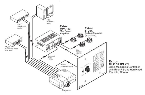
Application diagram using an MLC 52 VC with an MPA series power amplifier
